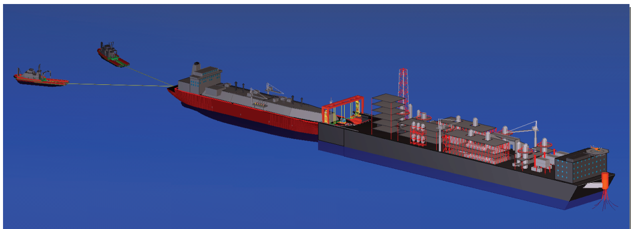
Figure 1: Illustration of the new proposed offshore LNG transfer system with the LNGC berthed in tandem configuration to the 'mooring bay' at the LNG terminal
