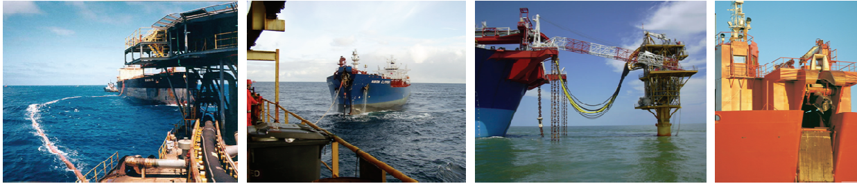
Figure 2: Tandem mooring configuration for standard offshore crude oil transfer, using floating and submerged hoses; fishtailing movements of the shuttle tankers moored to FPSOs (both left); bow loading systems (right) (Sources: Kongsberg, APL)
