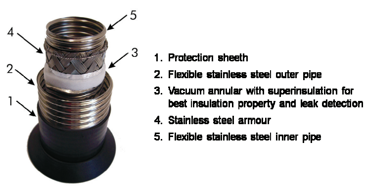
Figure 5: The LNG transfer pipe system CRYOFLEX offers a newly developed design with 16-inch inner diameter
