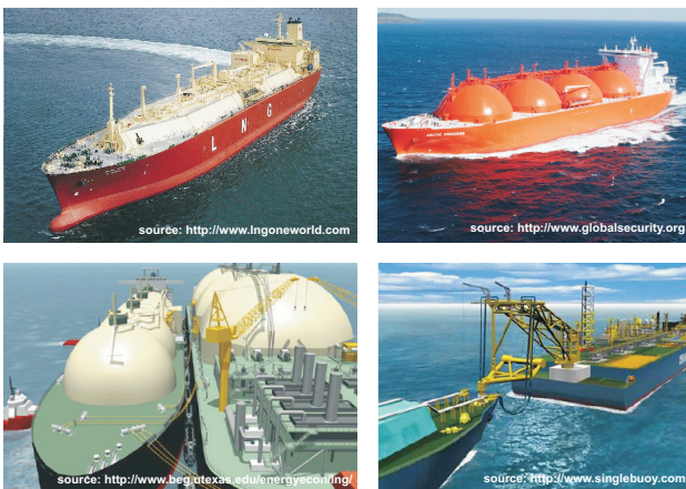
Figure 2. LNG-CARRIER WITH MEMBRANE TANKS (TOP LEFT), AND SPHERICAL 'MOSS' TANKS (TOP RIGHT), IMPRESSIONS OF OFFSHORE LOADING IN SIDE-BY-SIDE (BOTTOM LEFT) AND TANDEM CONFIGURATION (BOTTOM RIGHT)
