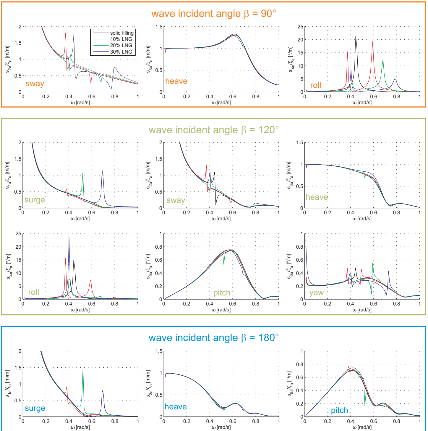
FIGURE 8. COMPARISON OF RAOs FOR DIFFERENT LNG FILLING LEVELS AND WAVE INCIDENT ANGLES OBTAINED BY WAMIT
