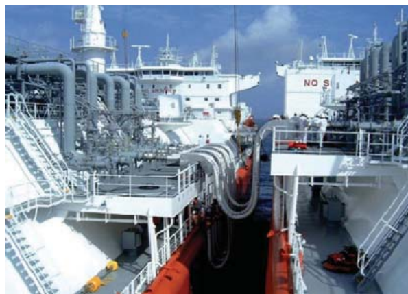
Fig. 2: The Exmar / Excelerate Energy Bridge uses composite hoses for LNG transfer in side-by-side configuration (Source: TNO)
