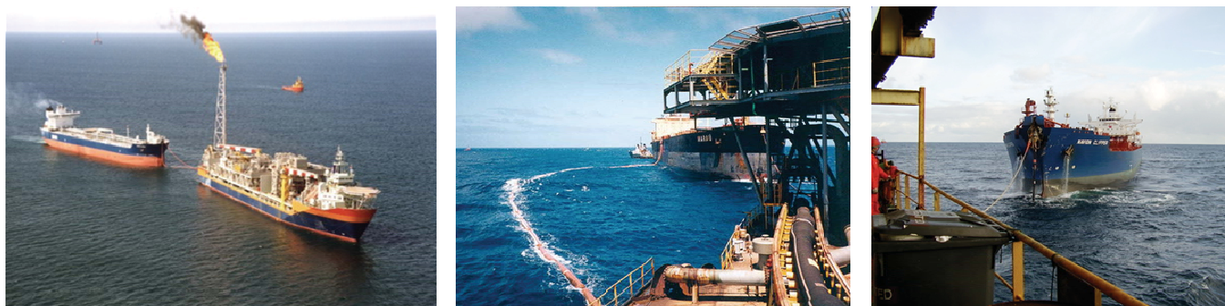
Fig. 3: Tandem mooring configuration for standard offshore crude oil transfer, using floating (middle) and submerged (right) hoses, with fishtailing movements of the shuttle tankers moored to the FPSOs (Sources: Kongsberg, APL)
